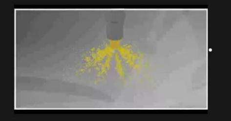
The injection system must atomize fuel for it to combust, so the spray nozzles have either a single hole near the tip or a series of holes around the side.
