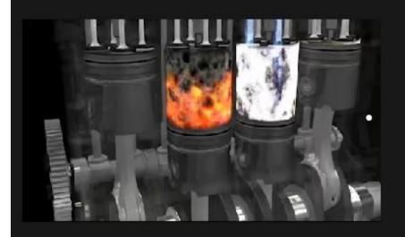
As with air and exhaust valves, Cummins fuel systems use the camshaft to control the injection process. The amount of fuel delivered to the cylinder is controlled in part by the speed at which the engine turns, since the camshaft is connected to the crankshaft.
